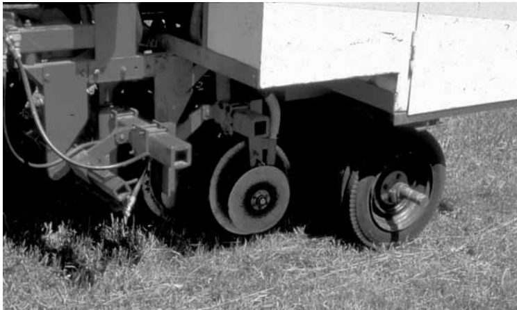
Left: Coulter-type disc drill used by Dr. Malhi to band P below the soil surface in established alfalfa stands.
